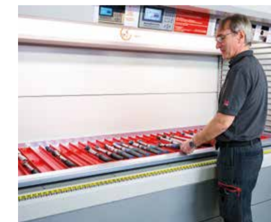
At Fill, a store keeper collects all operating equipment from the lift system.
